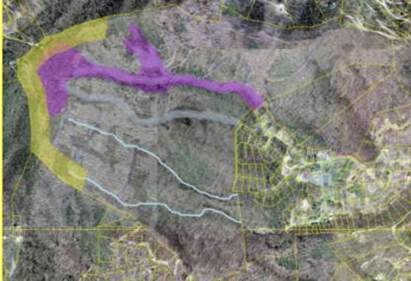
A Tier 1 SRA showing basic analysis of existing conditions (aerial photography), streams, drainage ways, poor soils and an important ridgeline using information from a brief field visit and commonly available GIS data.
